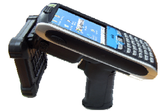
Rugged handheld scanner with GPS, RFID and barcode reader, digital camera, and wifi/cell phone connectivity
